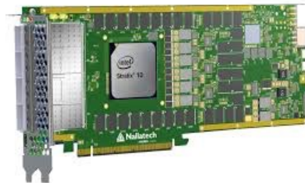
BittWare 520N with Intel Stratix 10 FPGA equipped with 4x 100Gbps optical interconnection interfaces
