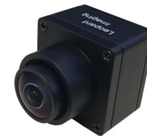
Leopard Imaging w/ FlickerMitigation (Camera / Traffic Light Recognition)
