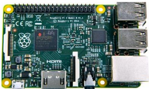
Broadcom 2836 900 MHz quad-core ARM Cortex-A7 CPU
